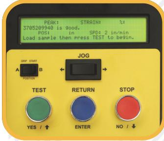
Backlit LCD screen shows peak poundage as well as test speed and elongation.
