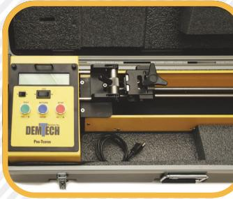
Unique grip design for 1 inch (25mm) coupons and 4 inch (100mm) "grab" tensile tests.
