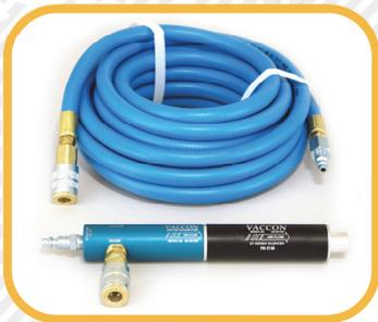
The Ventury Kit is used attached to an air compressor to convert air pressure into vacuum to supply all non self-contained models. The attachment provides up to 20 inches of Hg (10psi).
